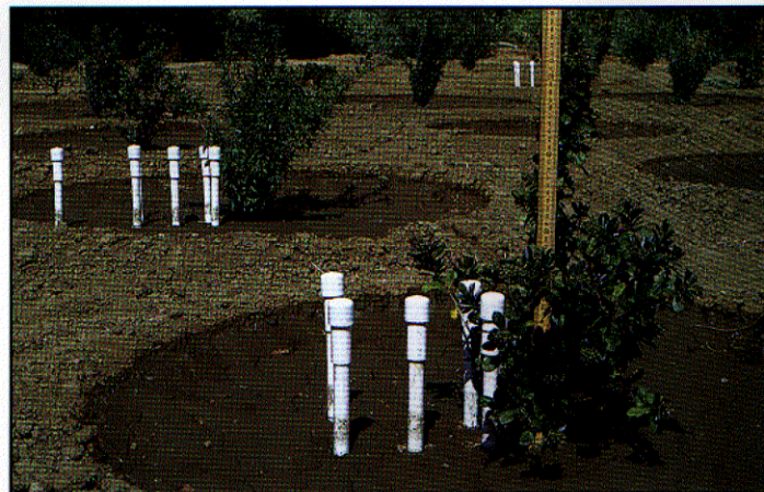
Apparently healthy container-grown plants often do poorly when transplanted. Tests with privet at UC Davis showed that, for best establishment and plant growth, frequent irrigation is vital to achieve maximum root development of a newly transplanted plant. The pipe-like devices are tensiometers, which measure soil drying patterns.
