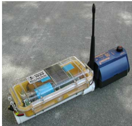
Figure 2. Third generation valve controller with 1-inch latching valve.
